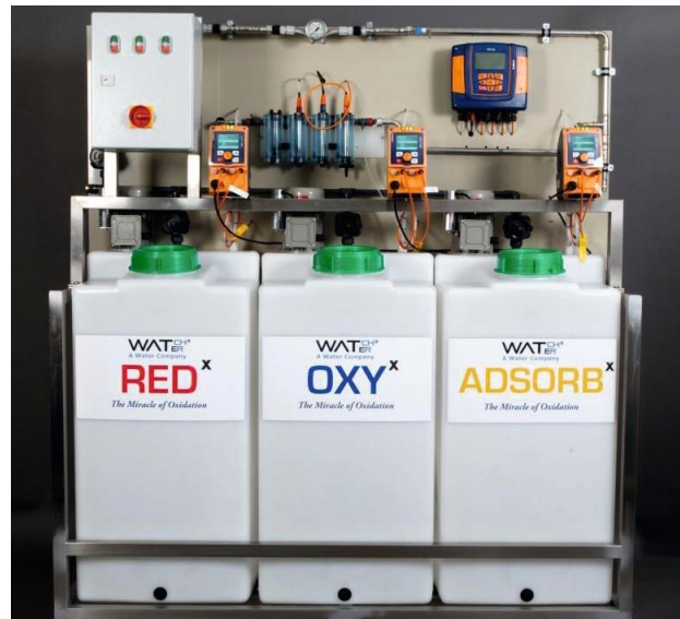
A real prototype of RED-OXY ® Dosing system (made by Watch-Water ® Germany)
