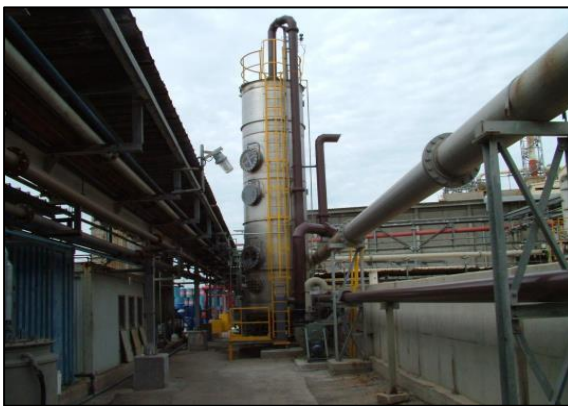
Two-step bio-trickling filter (BTF)
