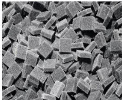
Figure 1. Delivery form (20x20x7 mm) of LEVAPOR and cross-section (magnified)
